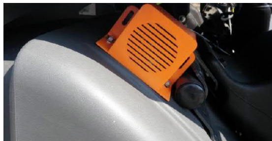
Figure 6: Vehicle manoeuvring warning for left-turning
